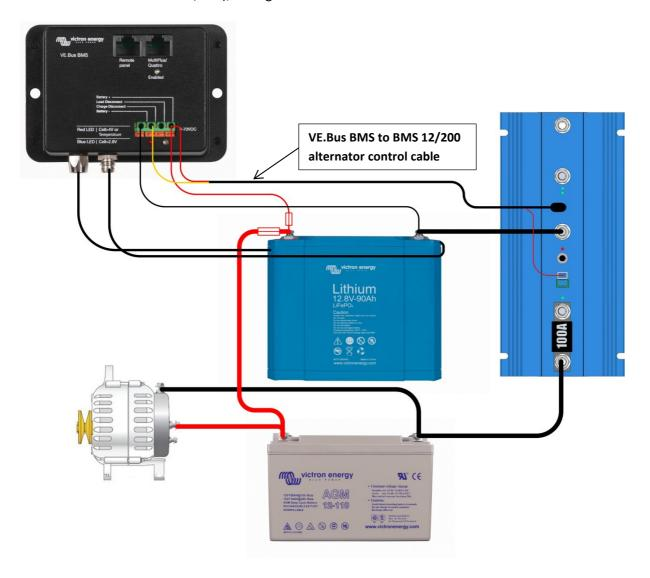
NOTE 1: The Li-ion battery and any loads powered by the Li-ion battery must <u>not</u> be connected to ground.
